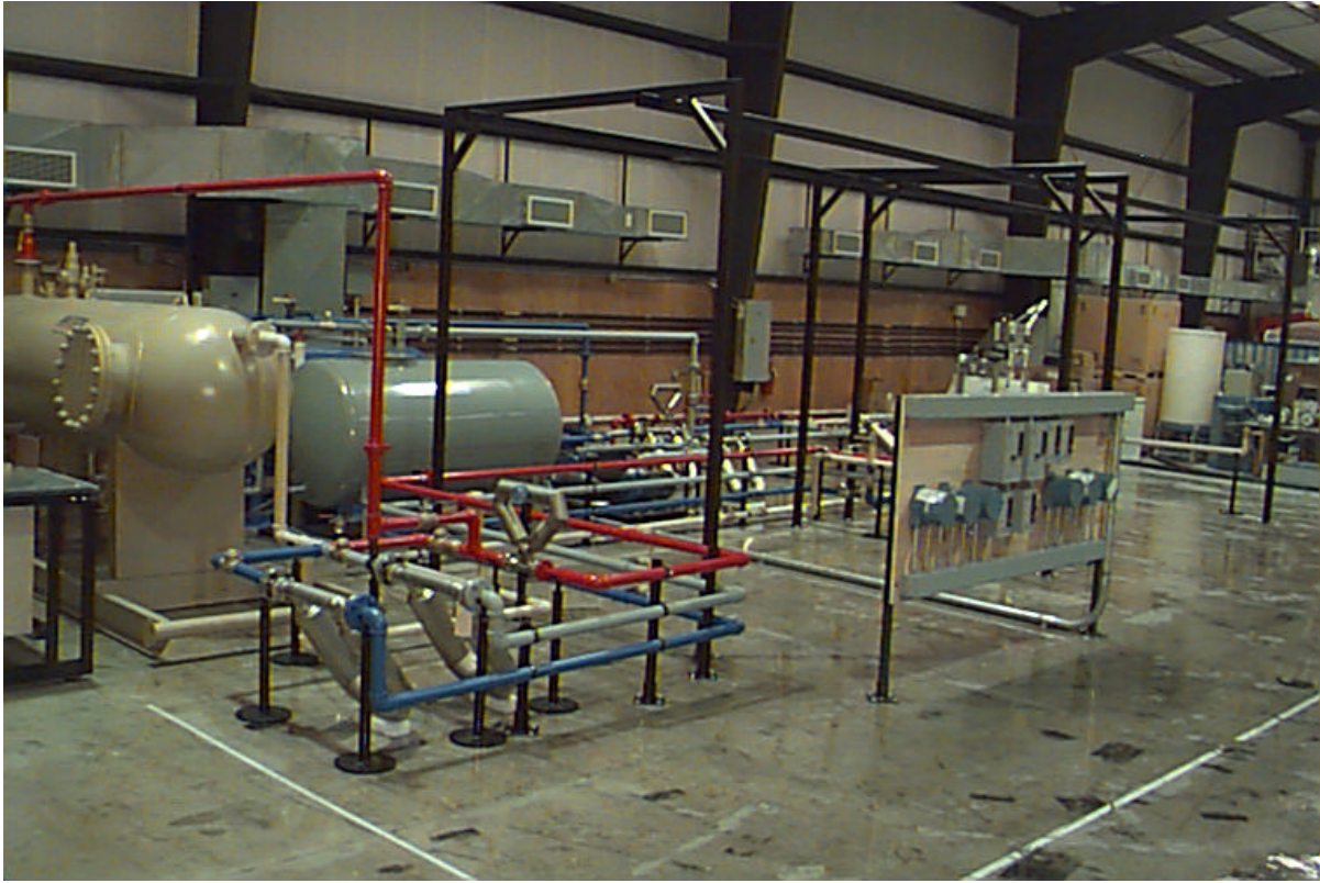
Figure 1: TUSTP New DOE Three-Phase Flow Loop Facility
